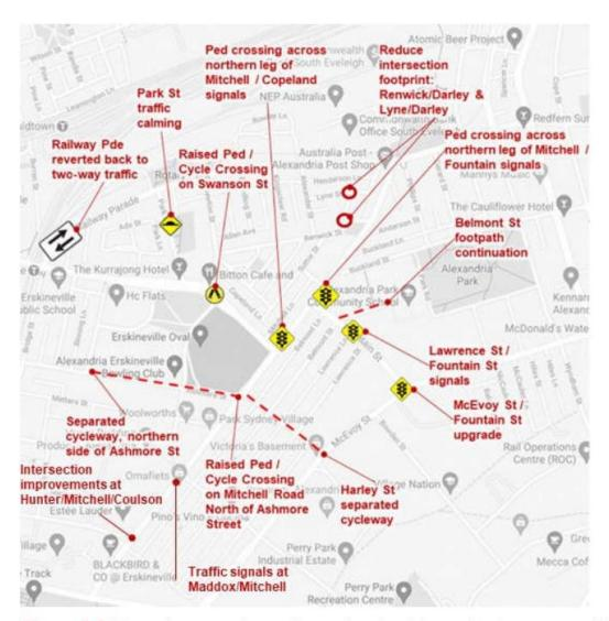
Figure 1.2: Base Assumptions: Committed or Recently Constructed Works
